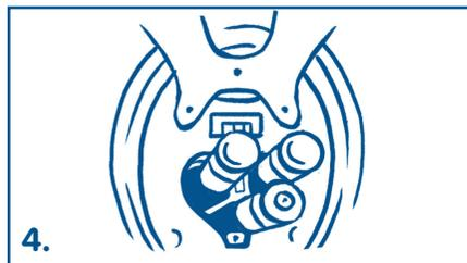
4. Replace with three new 1.5 V "C" size alkaline batteries. Be sure to orient the batteries correctly as noted in the duck's battery compartment.
