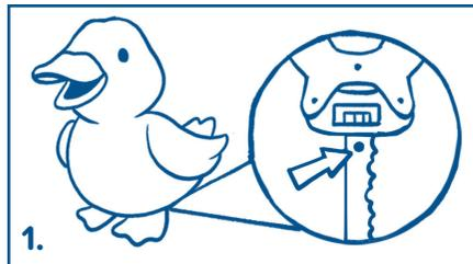
Locate the button-like screw near the power switch.
