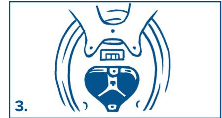
3. Remove the cover and all of the batteries. Discard the old batteries.
