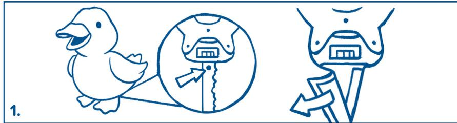
1. Loosen the button-like screw behind the duck's feet and undo the hook-and-loop fastener. You should see the battery cover.
