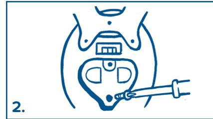
2. Use a Phillips/cross-head screwdriver to loosen the screw in the battery cover.
